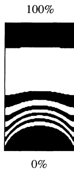
FIG. 12. Typical concentration map as given by the computation ( \mathcal{D}=5 \times 10^{-3} ). The alternate black and white stripes correspond to C_\infty/10 concentration intervals. The concentration is set to zero in the rear part of the branches (see the Appendix). Tips are at the bottom corners of the picture.
