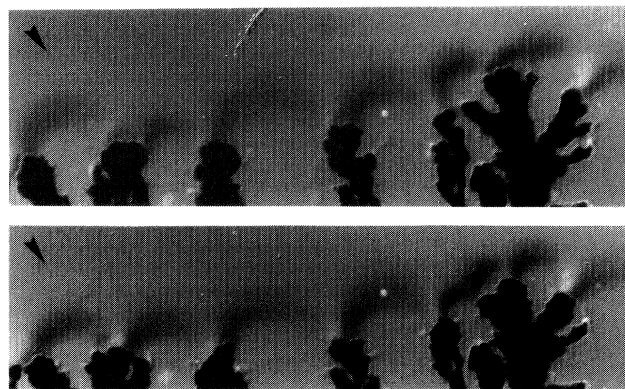
FIG. 17. Two consecutive images of the concentration gradient obtained with the interferential contrast (see text) on an almost steady growth. One should view the contrast on the pictures as the shadow of the concentration profile, with a spot light coming from the direction of the arrow. The concentration is 5 \times 10^{-2} \text{ mol l}^{-1} , a potential of 8 V was applied, the cell geometry is 0.1 mm × 1 cm × 1.5 cm (because of using constant potential in this experiment, the growth is not in the steady state).
