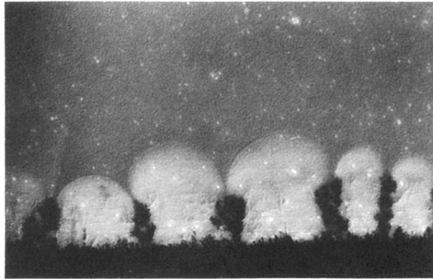
FIG. 19. Image of the convective vortices, just after the beginning of the growth. The darker aspect of the upper part of the picture is due to the very small oil droplets (diameter \approx 1 \mu\text{m} ) which are in the solution. The droplets hardly penetrate below the arch, because the fluid flow makes them drift through the funnel. (Same experimental conditions as in Fig. 17.) Note that the feet of the arches, where the tips are located, are very narrow: these are very active zones due to the high speed of the liquid going inwards.
